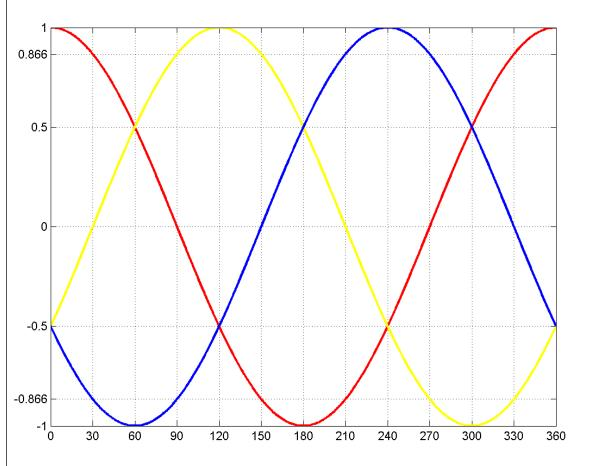
Rotating Magnetic Field  $B_{net}(t) = B_a(t) + B_b(t) + B_c(t)$
